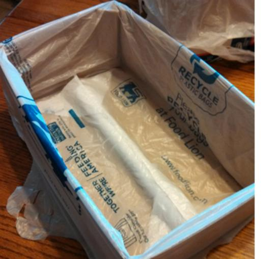
Line the box mold with some form of plastic, like a used shopping bag, over top of the channel.
