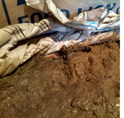
Firmly and heavily pack mix into paper rope sides.
